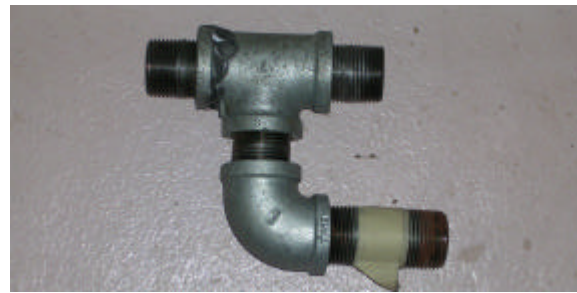
Figure 10. The mount is made from 1" plumbing fittings.
