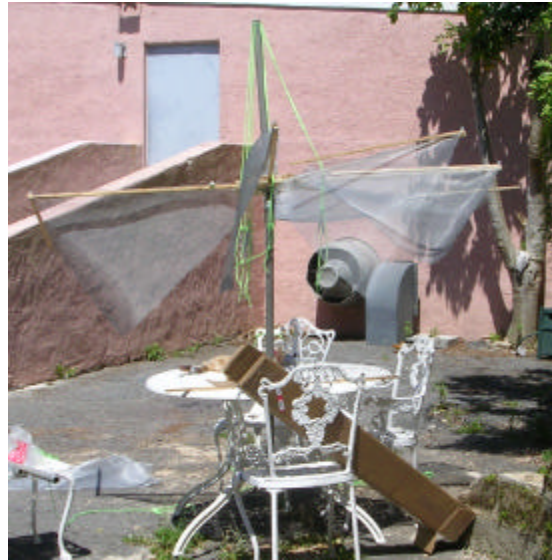
Figure 12. The spokes ( petals ) are attached to the center hub one at a time.
