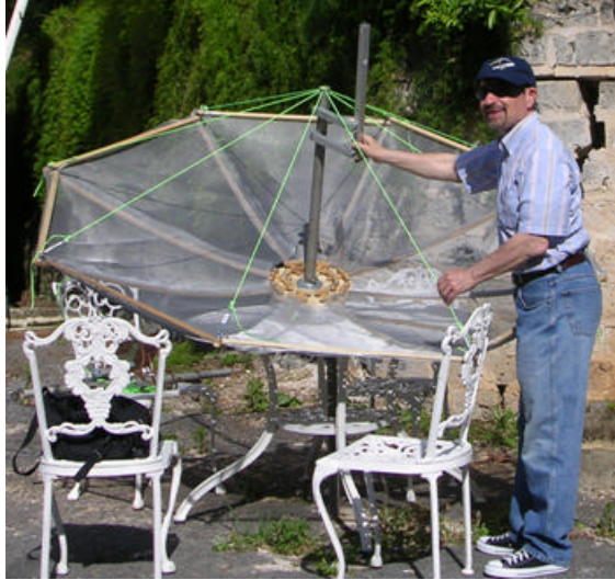
Figure 8. Installation of feed support.
