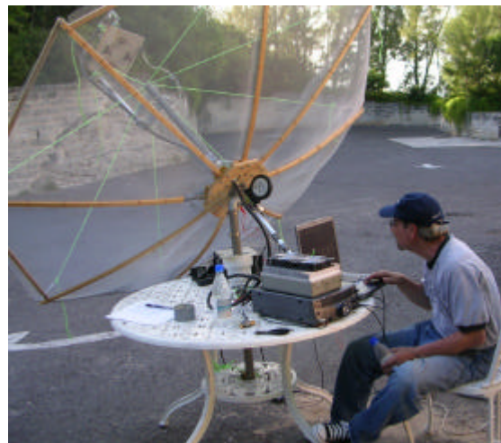
Figure13. Completed dish and mount.
