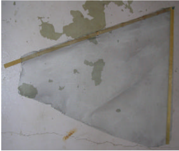
Figure 5. A petal is formed from a spoke , rim segment and aluminum screening.
