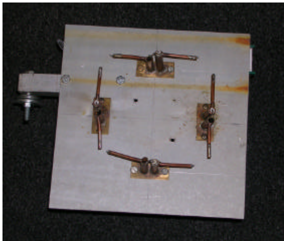
Figure 9. Dual dipole feed antenna.
