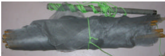
Figure 6. For travel the aluminum screening is rolled around the spokes and rim segments .
