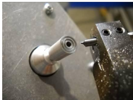
Fig 8 Tiny Multi Choke Ring dish feed Commonly known as a Chaparral™ (The centre hole is 2mm Diameter)
