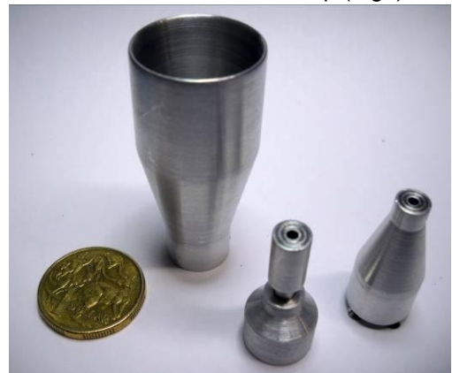
Fig 9 Horn, Adjustable and fixed feeds
