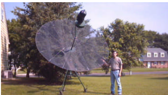
N2UO's 10' stress dish with feed in place
