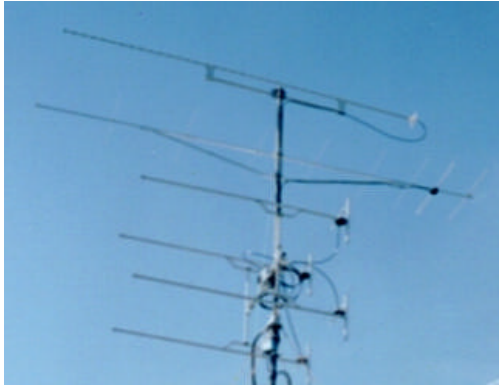
ES8X's 4 x 12 el yagi array (low part of picture)
