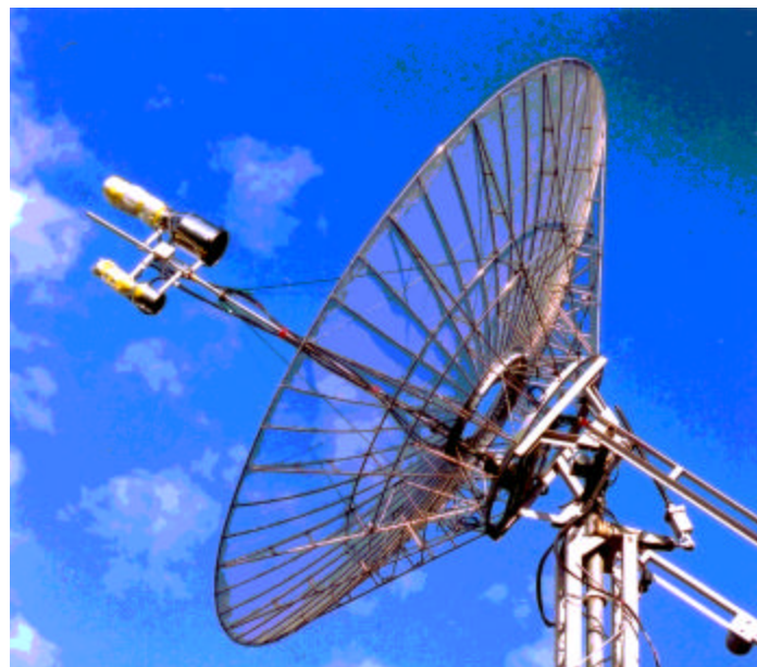
JA6CZD set for the EME contest on 23/13 cm with this neat mechanical feed switching arrangement. The dish is 5 m.
