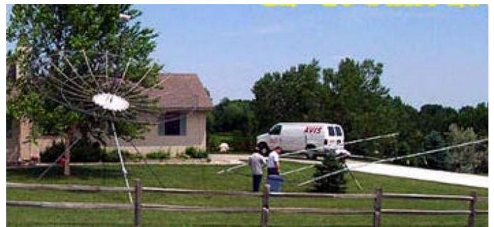
W2WD/0 Dxpediton site -- portable 20' dish for 70 cm.
