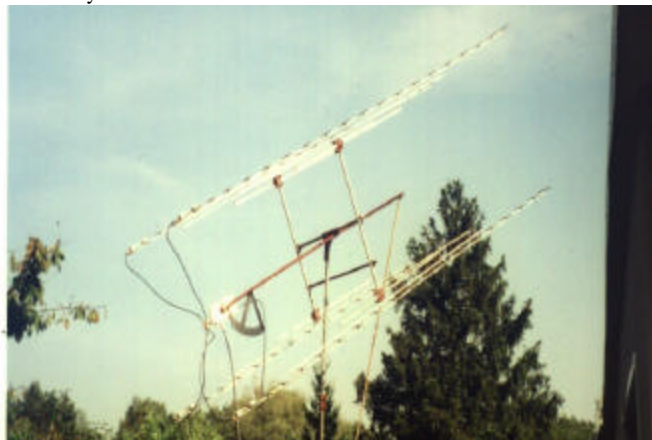
DL7UDA 4 yagi array with mechanical manual AZ-EL readouts
