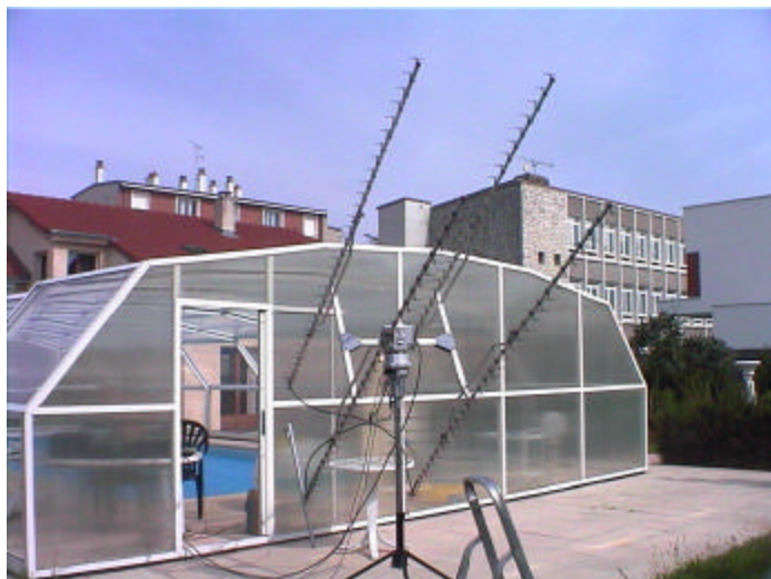
1296 JT44 echo test at F5SE using 4 Tonna yagis
