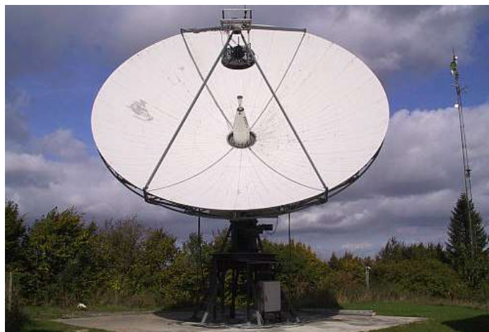
DL0SHF's 1296 9m Dish (Only SWL in Nov, 700 W to be on soon)
