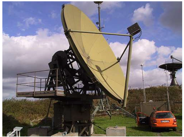
DL0SHF 3 cm Station (6 m dish and 350 w) – A separate 6 m dish was used on 13 cm!
