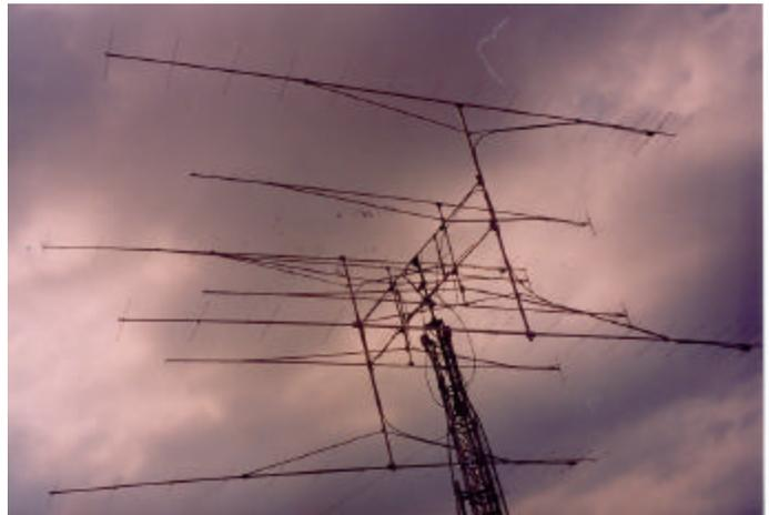
**YO4FRJ's EME Array - 432 yagis are inside 2 m array**
