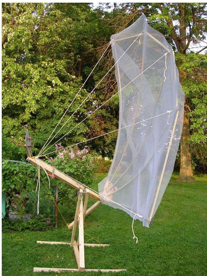
**7.5' offset stress dish for portable operation**
