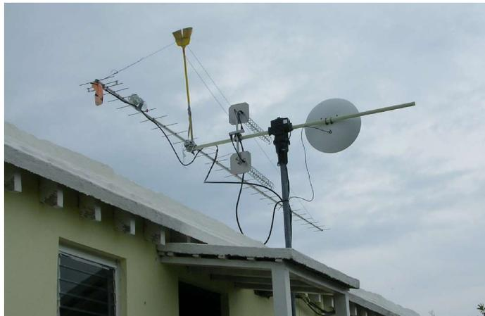
**VP9MU's antennas with yagi used for 70 cm EME**
