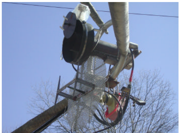
K2UYH's 1296 rotatable linear feed used with yagi stations
