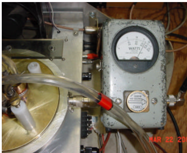
W2DRZ's 4 x 7289 PA (K2AH amp) showing ~ 900 W out (Bird slug is 0.4 to 1 GHz and reads about 0.8 low. PA has 1450 Vdc on plate, current is 800 ma with 200 ma grid and drive is 40 W).
