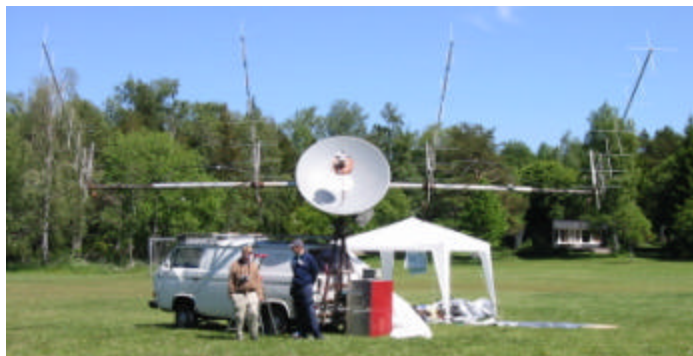
OH0/OH3MCK site with 1.8 m dish used on 23 cm
