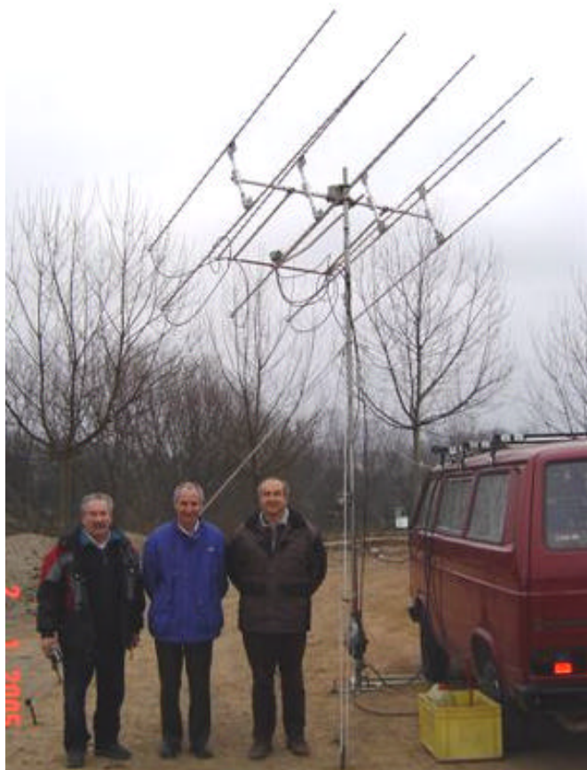
EA3BB Test Team with 23 cm 8 Yagi Array
