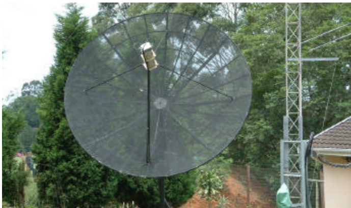
ZS5LEE 1296 cm 3.8 m dish with OK1DFC Septum feed
