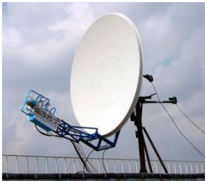
RW3BP's 2.4 m offset dish and 47 GHz system
