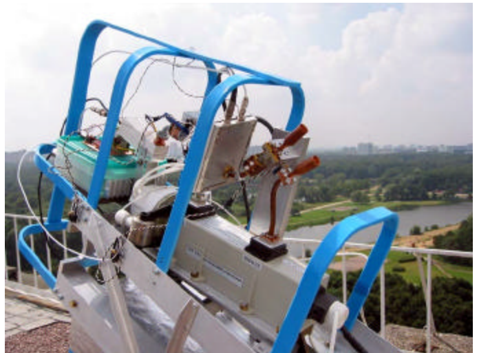
More details of RW3BP 47 GHz station – note dual feeds used for RX & TX
