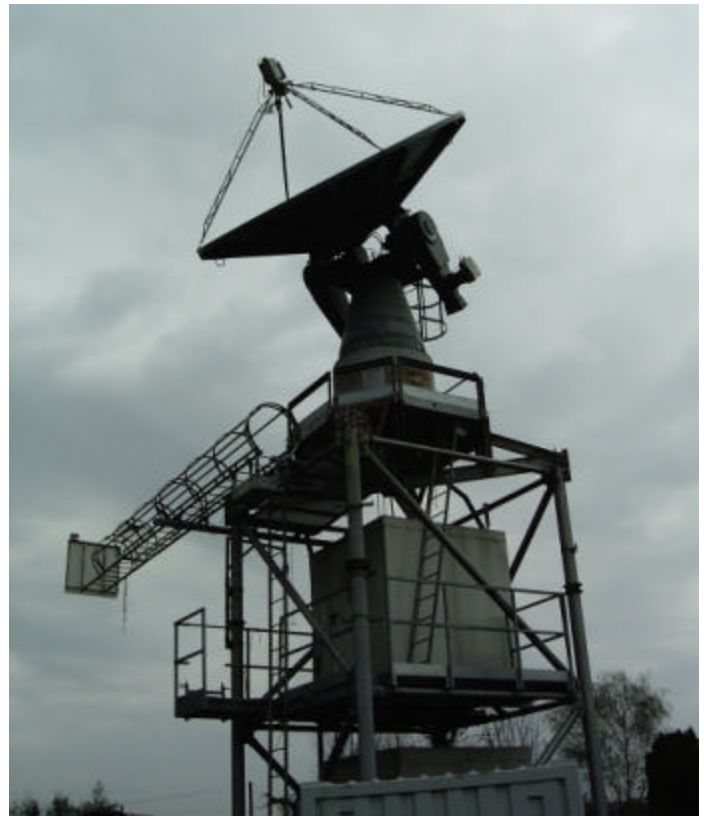
OK1KIR's new 4.5 m dish with TWTA mounted at rotatable linear feed
