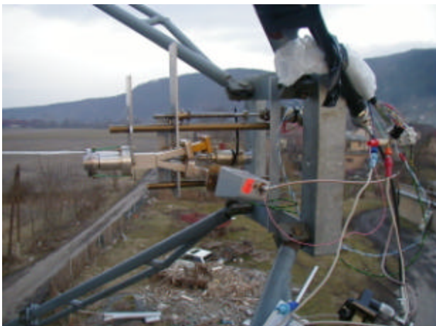
OK1KIR's 10 GHz feed arrangement
