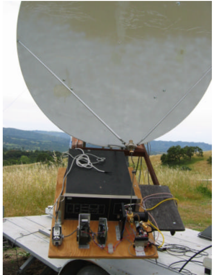
AD6FP's 1.8 m offset dish, 30 W TWTA & xvtr move with dish
