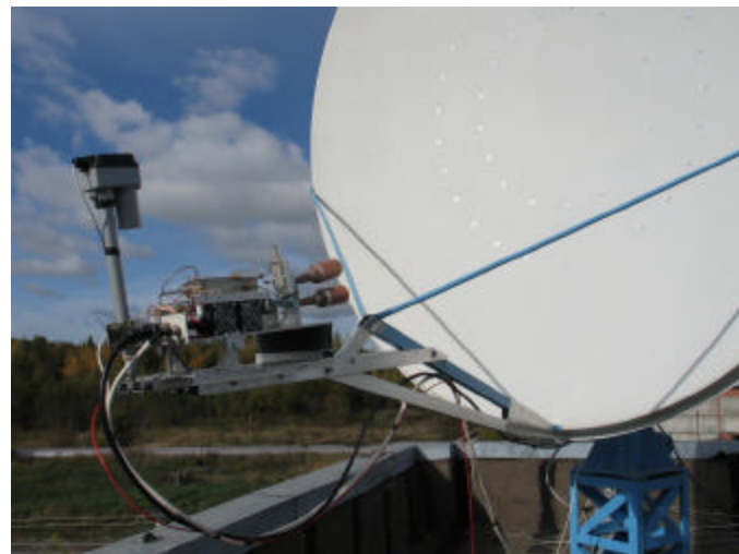
RW1AW 10 GHz dish and feed (see dual TX-RX feeds)
