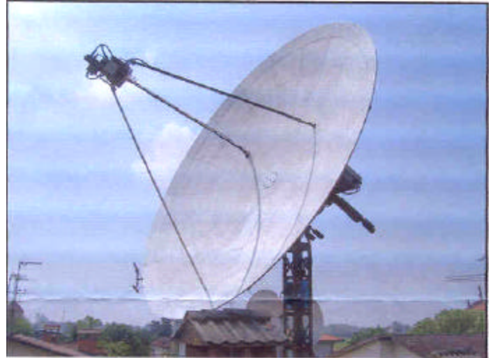
IK2RTI's 4.8 m dish made from 1.5 mm laminated Aluminum with 3 mm holes and 10 mm steps
