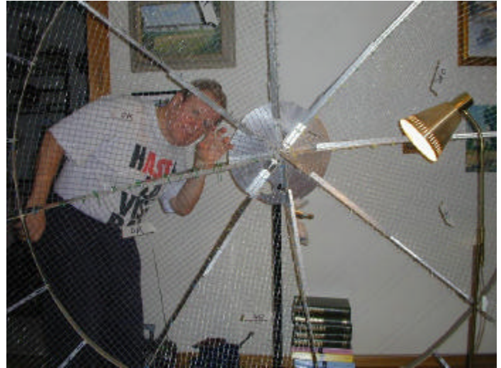
SMSLE working on his 2.2 m (9.9 kg) dish for 1296 EME
