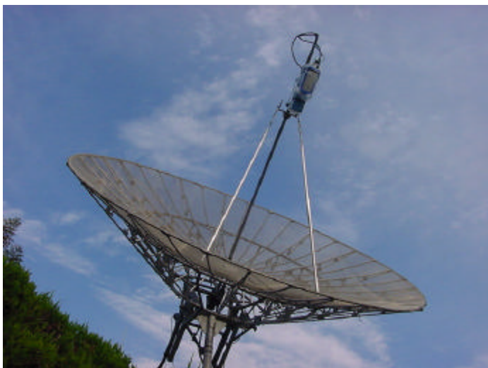
JA4LJB's 5 m dish with 100 w PA at Septum feed
