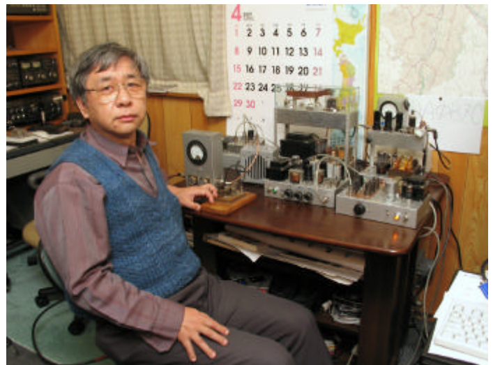
JA0BZC's all vacuum tube EME rig (on 2 m)
