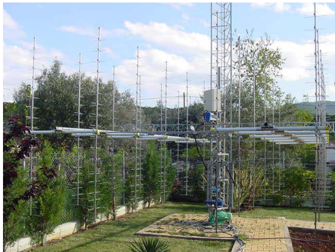
SV1BTR's new 24 cross pol yagi array – wow!
