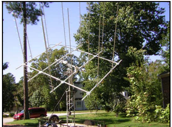
N8CQ's portable 12 x 16 el yagi array for 70 cm.
