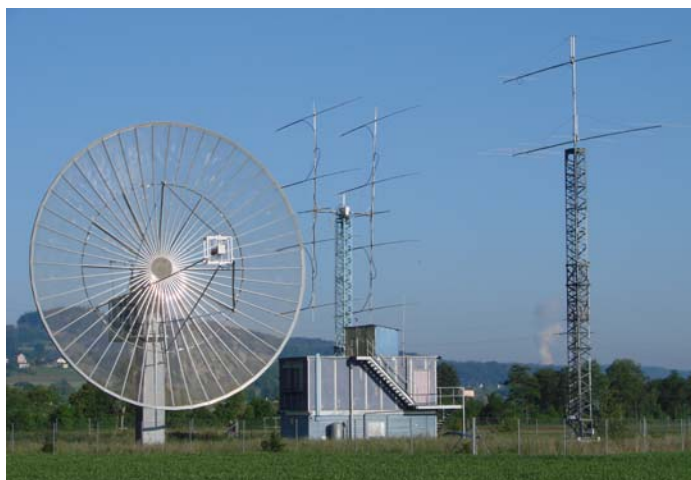
HB9Q's 15 m dish used on 70 cm for DXCC #2!
