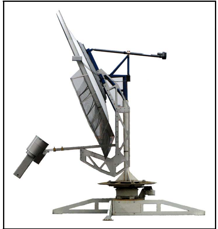
RA3AQ/RW3BP 2.4 offset dish used on 1296 for the contest
