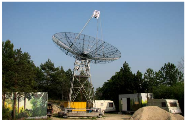
F5SE's new dish with feed in place and springs added
