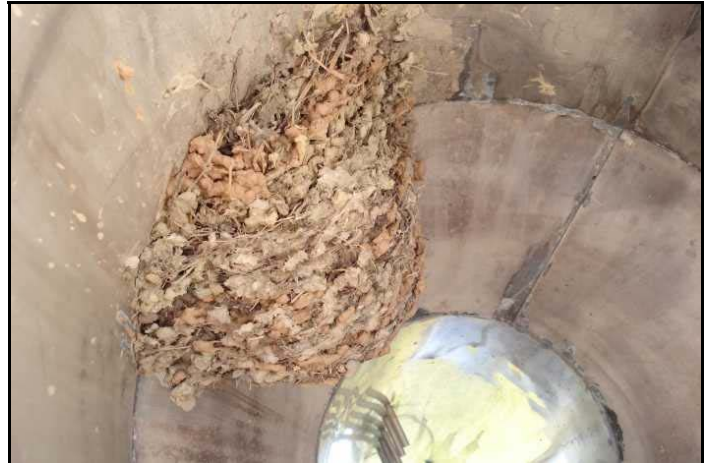
VK3UM's horn feed with Swallows nest – Does wonders for the VSWR!
