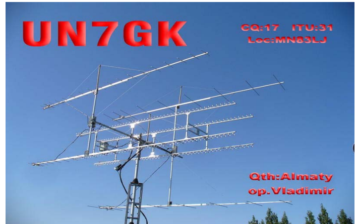
UN7GK's EME arrays for 2 and 70 cm
