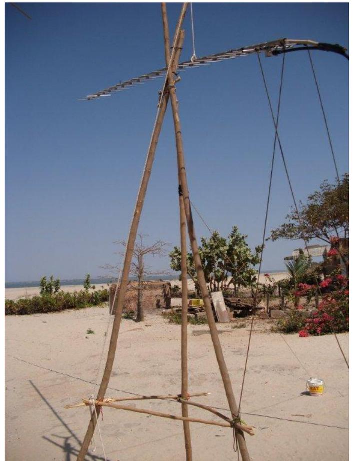
**C56EME yagi and locally constructed mount in Gambia**
