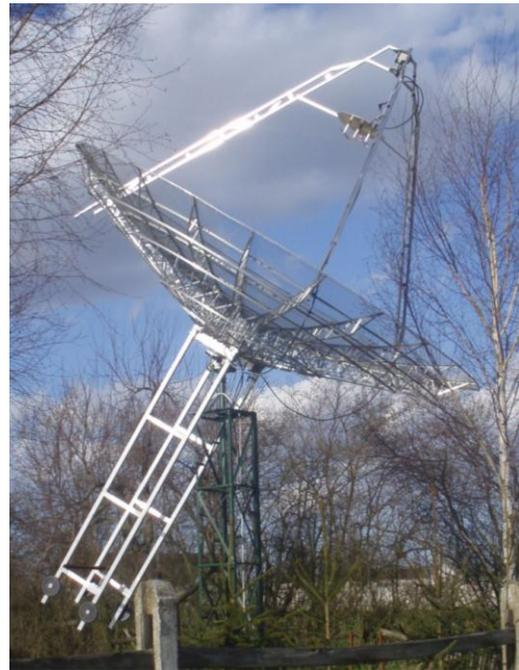
**SP7DCS's new 6 m with temporary 70 cm feed in place**
