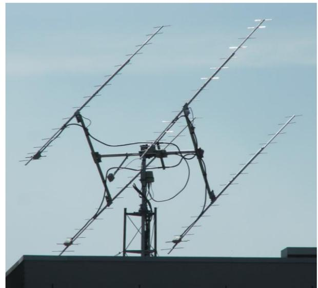
**PE1RDP's new 4 x DK7ZB yagi array**
