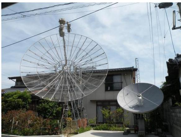
**JA4BLC** has two dishes (dish brothers) for use on L to K-band; L and S-band are on the 6 m dish, and an X band feed on the 3 m dish.
