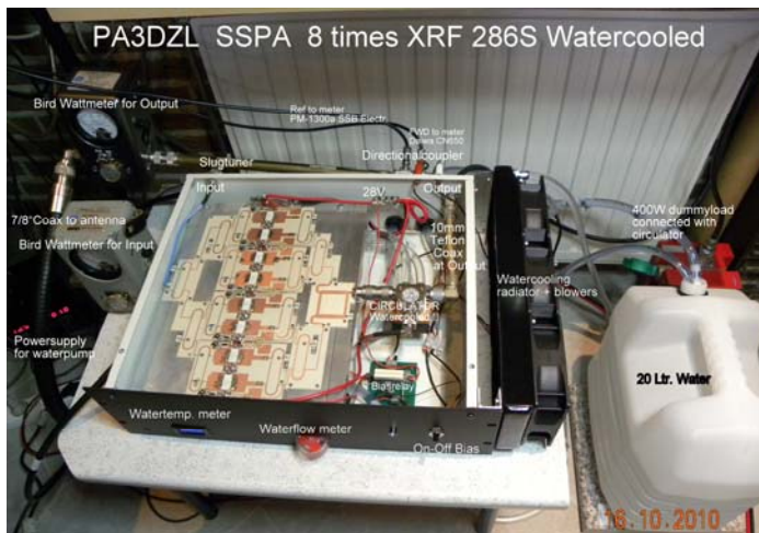
PA3DZL's water cooled 23 cm SSPA
