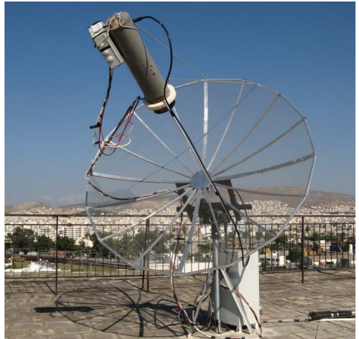
SVICAL's 2 m dish with septum feed and 45 W SSPA
