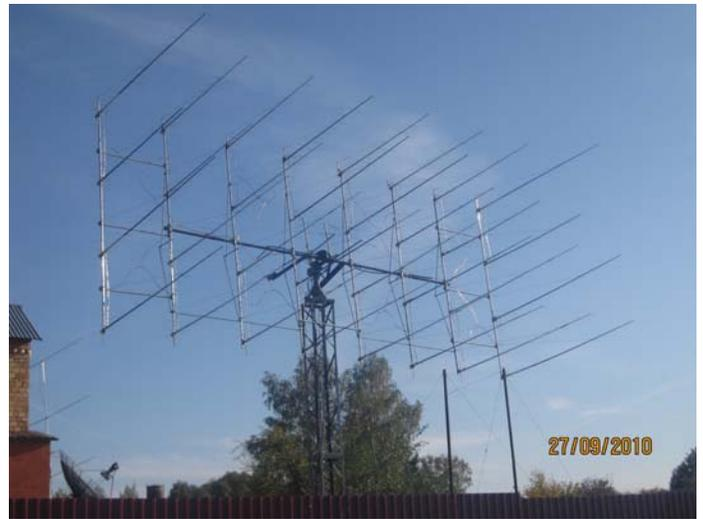
**UA3PTW's 24 yagi array used on 70 cm (23 cm dish lower left)**
