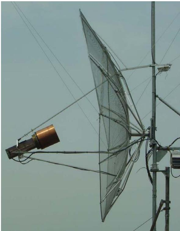
**OE5JFL's partially offset dish or how to turn a 2.8 m dish into a 3 m dish**
