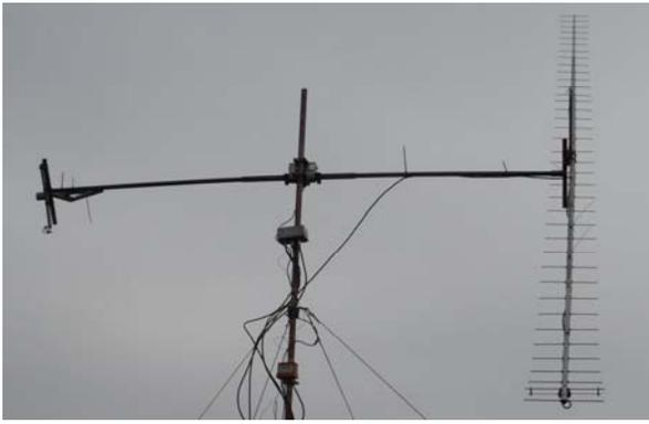
**DL5MAE used a 38 el M2 yagi on 70 cm in Nov**
