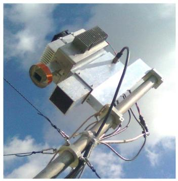
OK1CA's 13 and 6 cm multiband feed arrangement
