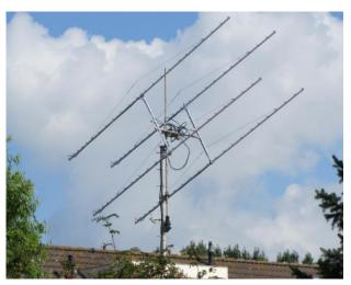
PA2V's new 4 x LFA yagi array
