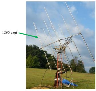
K3MF's yagi for 23 cm EME was mounted on his 70 cm array
