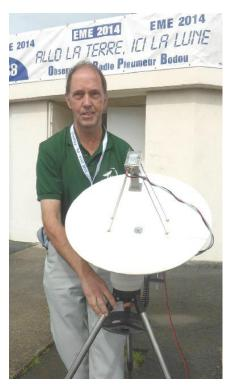
PA0EHG with 0.5 m used to demo 10 GHz EME
