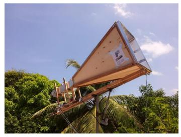
HK1H 0.8 m on a side horn used on 1296 EME
