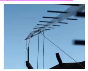
5B/PE1L's 67 el yagi used on 1296 to make 27 QSOs
