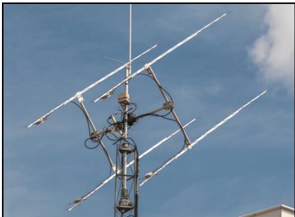
PE1RDP's 4 x 5.5 WL DK7ZB yagi array
