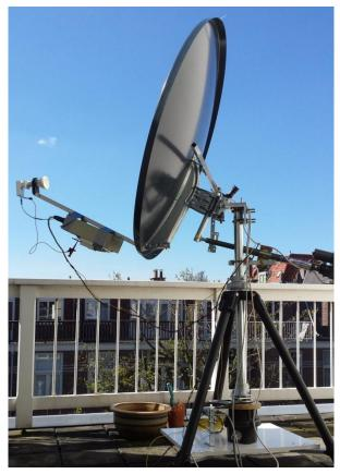
PA0HRK's 3 cm station using 1 m offset dish
