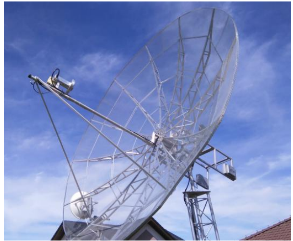
OK1YK 4.5 m dish & 13 cm feed [source ok1yk.blogspot.com]
