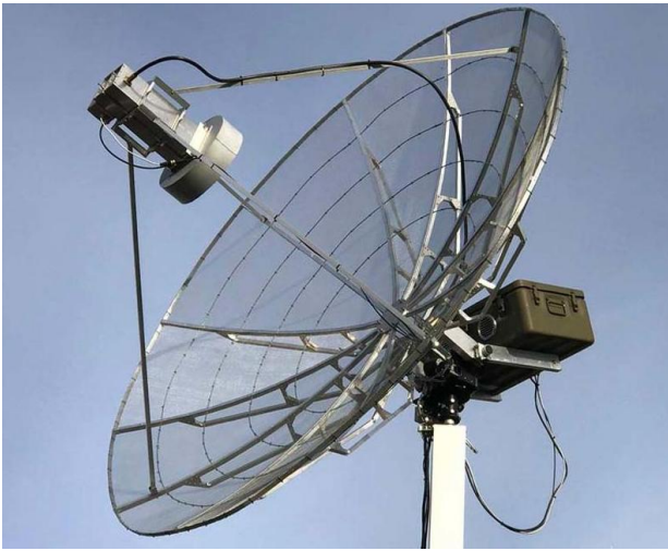
OK1IL's 3m EME mesh dish from Rfhamdesign
