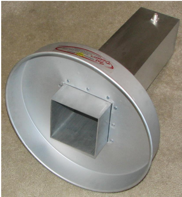
KL6M's cake pan scalar ring for 1296
