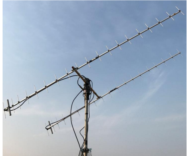
BV3CE's 2 yagi array for 432 EME
