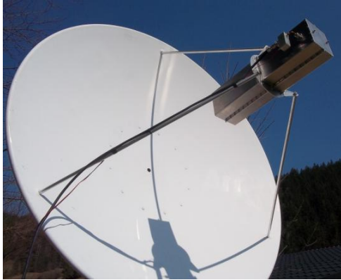
OK2PE's 1.8 m solid dish used for his first QSOs on 23 cm EME
