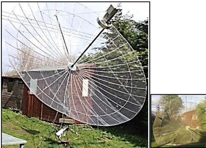
G4RGK rebuilt dish – damaged dish shown at right
