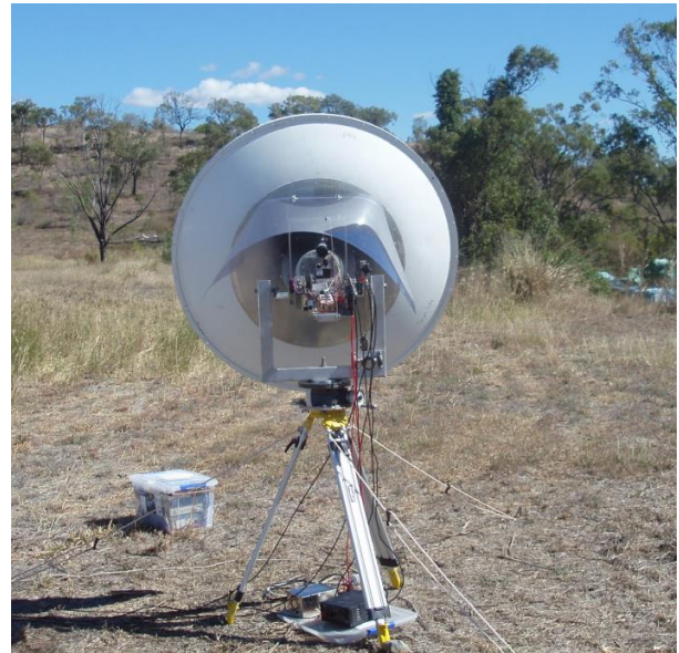
VK7MO's grid square dxpedition 3 cm setup with 113 cm dish and 90 W
