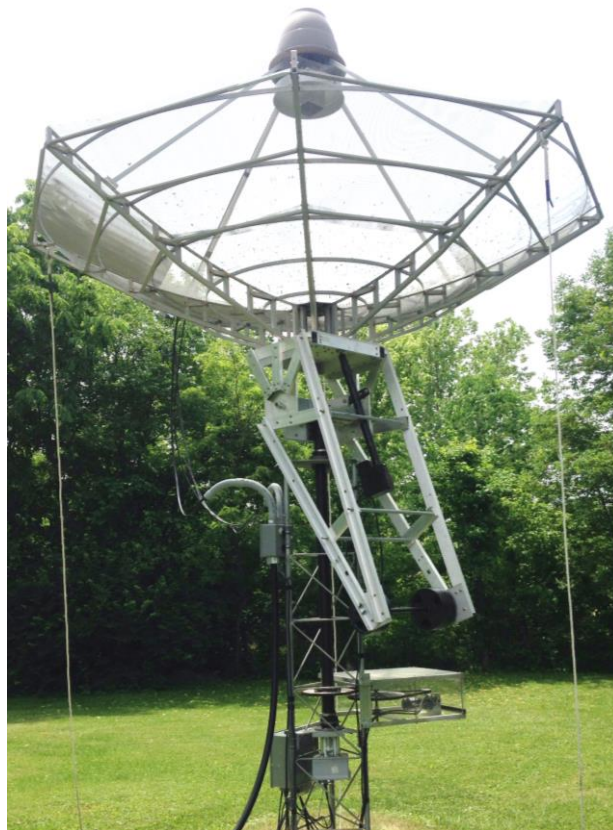
WB8HRW's 3.8 m dish used on 1296 EME
