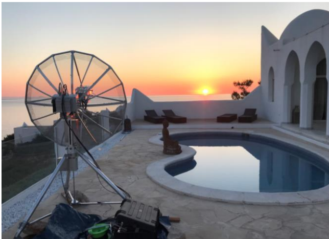
EA6/HB9COG's dxpedition QTH with 1.5 m dish and 13 cm feed at moonrise
