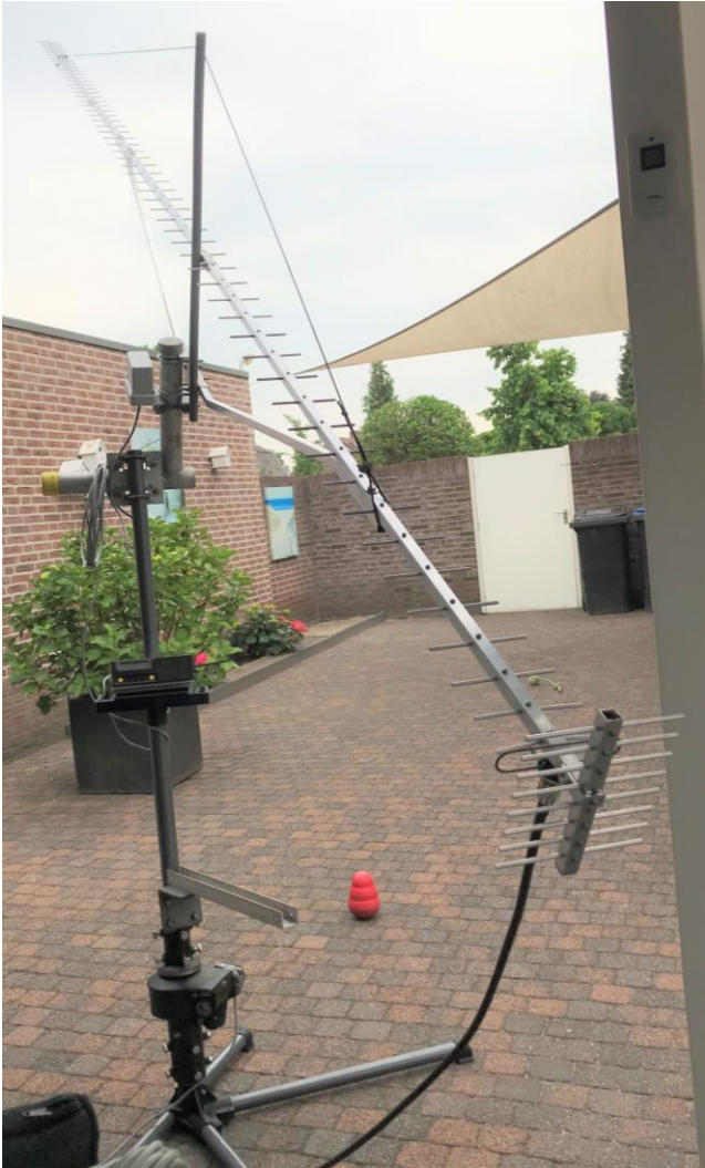
PA3DZL's temporary EME station being used while moving QTHs – on 1296 67 el yagi and 120 W
