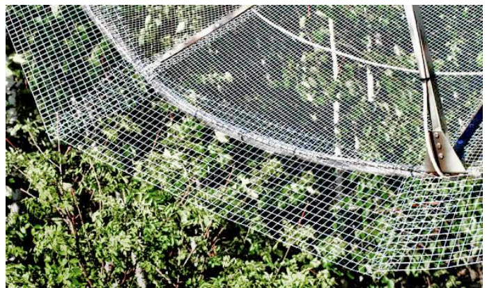
KA1GT's simple hardware cloth dish extension ~+1 dB
