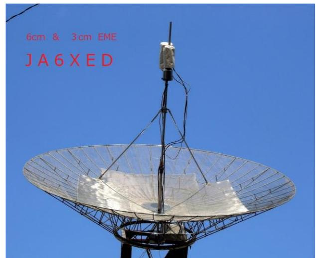
**JA6XED 5m dish with added fine mesh for 3 cm EME**
