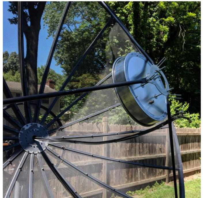
**W2HRO's 432 Cake Pan feed [Based OK1DFC's feed design but using a standard available cake pan to ease construction]**
