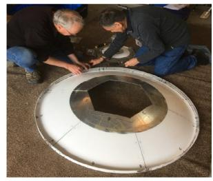
Roger ZL3RC (left) and Rex VK7MO (right) assembling the 1.13 m flyable dish. This was cut-up from a sold aluminum dish with a jigsaw - [See also Oct NL page 7].
