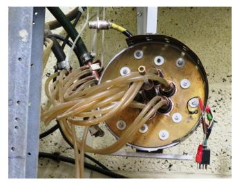
G3LTF's 6-tube ring PA suspended by cooling lines
