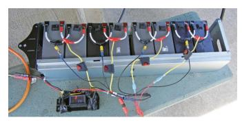
W5RZ's bank of 7.2 A/h sealed lead-acid batteries
