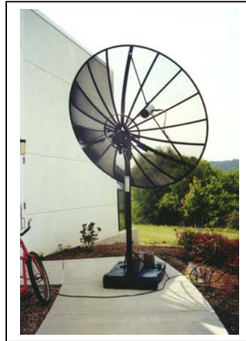
Spectral Hydrogen captured on a 7.5' diameter Antenna (Carl Lyster at NRAO)
