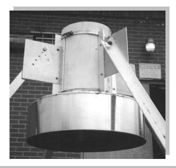
Feedhorn secured within a split, six inch PVC pipe. Fabricated aluminum brackets have been attached to the PVC pipe by adjustable ring clamps. Feedhorn supports are connected via ¼ inch bolts. Notice the additional holes for fine adjustment.
