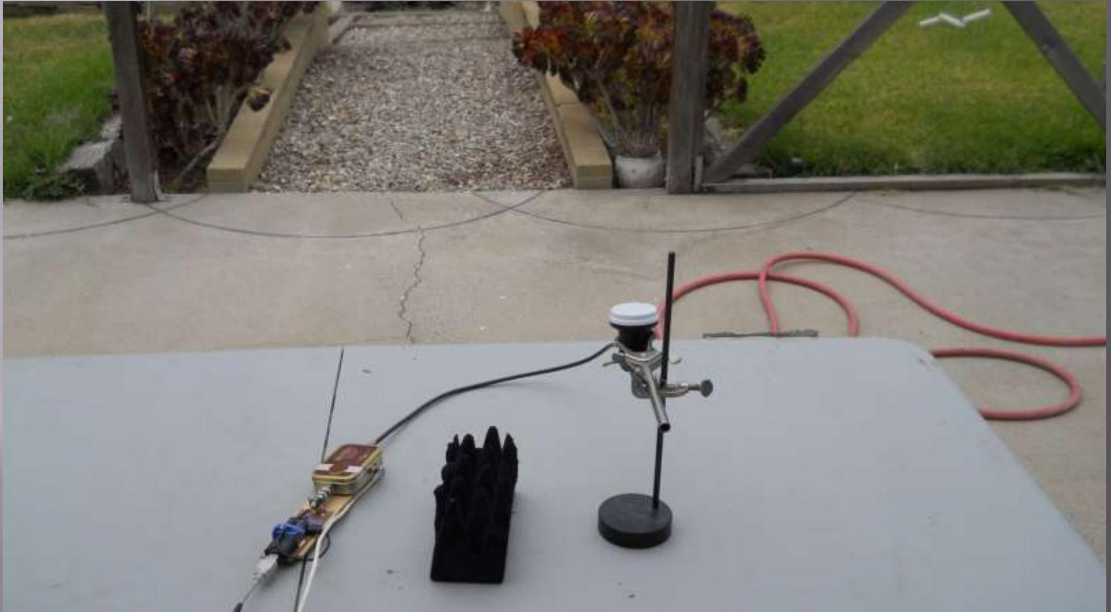
Rein takes advantage of the excellent front-to-back ratio of the Ku band feedhorn to reject ground noise. Plus it is pointed as far away from the ground as practically possible.
