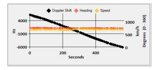
Contrast the geometry just described with the Doppler display shown above, obtained from a plane that was flying perpendicular to the direct path between the Home and DX stations. Note that the Doppler shift ranges between +6000 and -6000 Hz, and both the shift and its rate of change are far greater than the values shown for the aircraft flying down the inter-station path.
