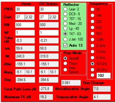
To perform the RF calculations for a selected aircraft, the user first selects the desired aircraft by left-clicking on it, and then selects in the section labeled "Reflector" (see the image on the left) the plane size category (Lear, DC-9, 707, Med, Lg, 747,or J Jet) by left-clicking the appropriate radio button. These select RCS values of 2, 8, 16, 20, 40, 63, and 100 sq. m respectively.
