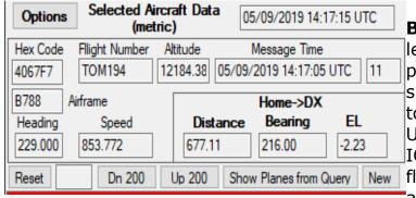
Basic Plane Data Area On the left is an image of the topmost portion of the data area on the left side of the main form. At the very top it shows the current time in UTC. Just below that, it shows the ICAO hexcode for the plane, its flight number, altitude, and the time at which its data was received. Just
