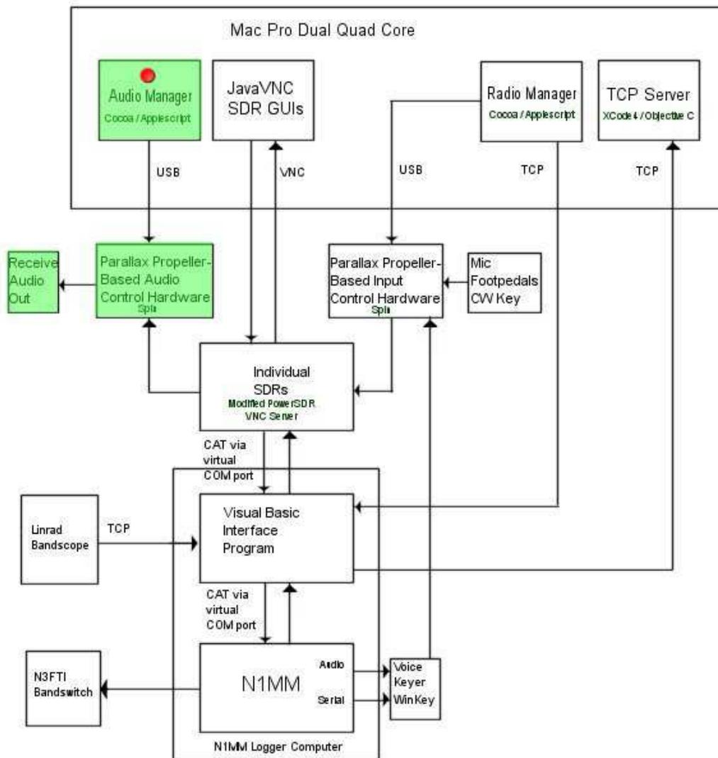
Thus one can at any time select a radio/band and frequency from either the GUIs on the Mac Pro or from N1MM. Any change or selection made at one location will be accepted by the other. For the operator, things function as if there is one 11 band radio with multiple bandscope coupled to N1MM by CAT control, with logging and all switching functions automatically controlled.
