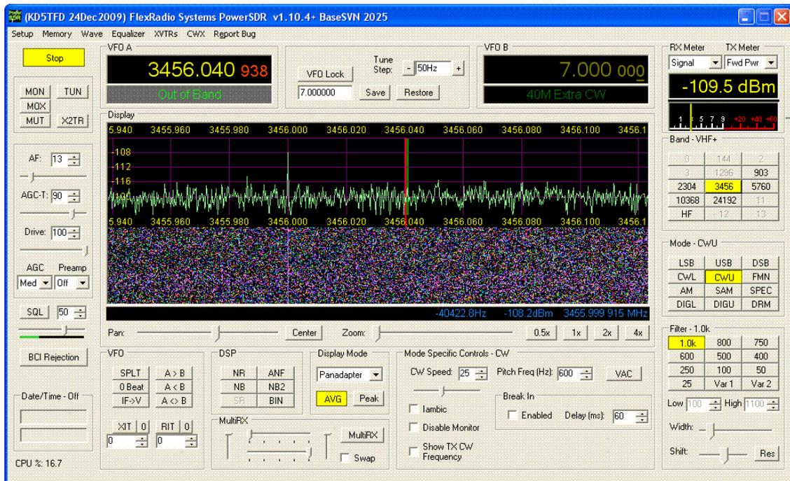
Below is a full width Large FFT size PowerSDR bandscope, same weak signal at 3456.041 MHz. Note that you can now actually see the weak signal on the waterfall:
