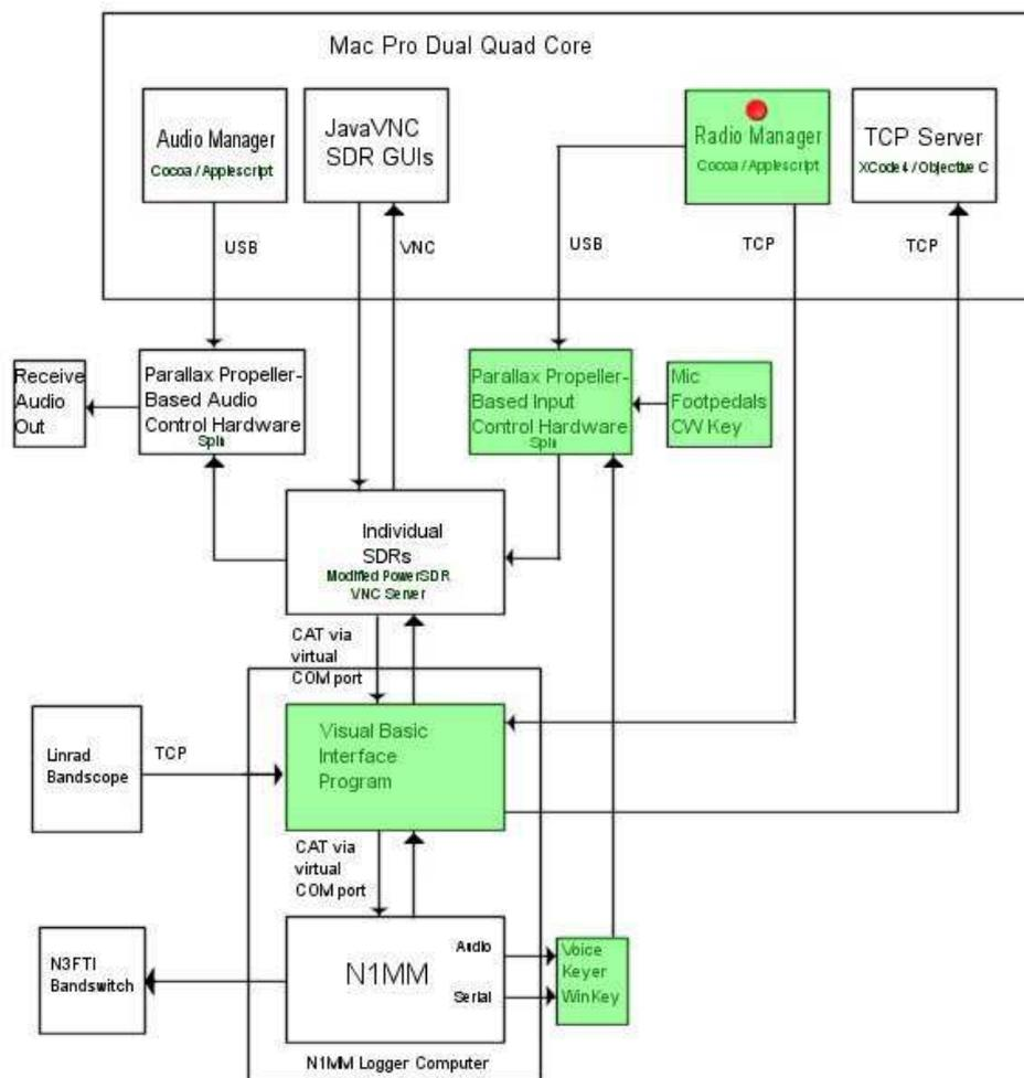
The Audio Manager is similar to the Radio Manager in that it also controls the homebrew hardware switcher, but its function is much more limited; it only functions to direct the received audio from the appropriate radios to speakers, headphones, or computer for the digital modes. It allows automatic or manual switching. Its place in the system is highlighted in green in the diagram below.
