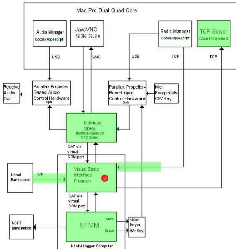
The logging computer also controls the antenna rotor via N1MM logger and a serial port, and WinKeyer, via N1MM logger and a USB-Serial Port adapter, and runs Win-Grid to serve as a check on the headings supplied by N1MM.
