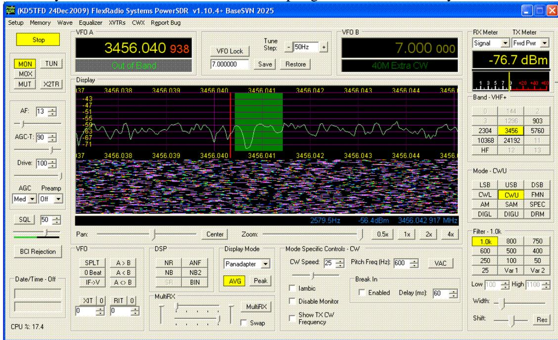
Below is the same zoomed-in spectrum with the Large FFT size version of PowerSDR. Note the smaller bin size, the superior frequency resolution, and the fact that you can actually see the signal (which is on the waterfall below and just to the left of the vertical bar)!:
