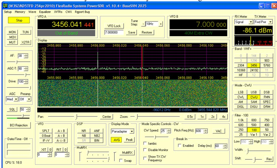
You can really see what the problem is with the standard FFT size PowerSDR when the bandscope is zoomed in below. The signal is again invisible and the large bin size that is forced by the small number of bins when sampling at 192 kHz is clearly demonstrated:
