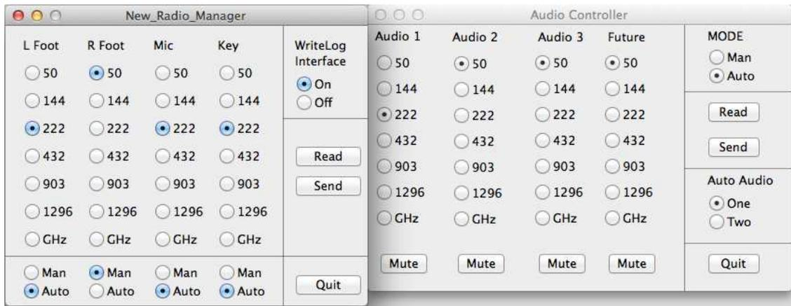
When on the microwaves, one footswitch and the microphone can be assigned to the liaison band, and the other footswitch and the key assigned to the microwave band, or vice versa, and a separate receive audio channel dedicated to each band.
