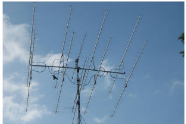
DL5FN's 8 x 9 WL M 2 yagi array for 70 cm EME
