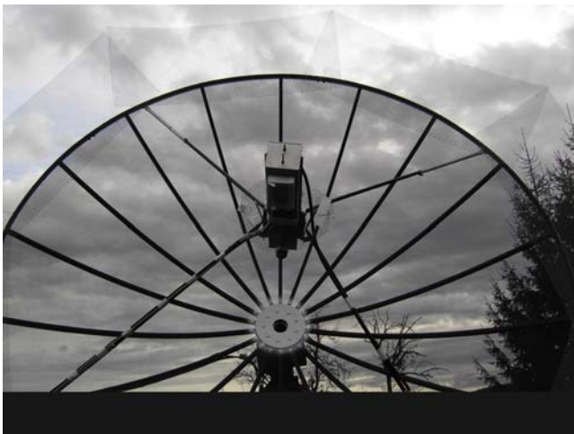
DL6SH's 3.8 m dish – note 12 mm mesh used to increase size
