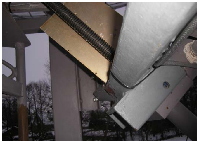
OZ4MM's Dish's bent bridge between the counter weights
