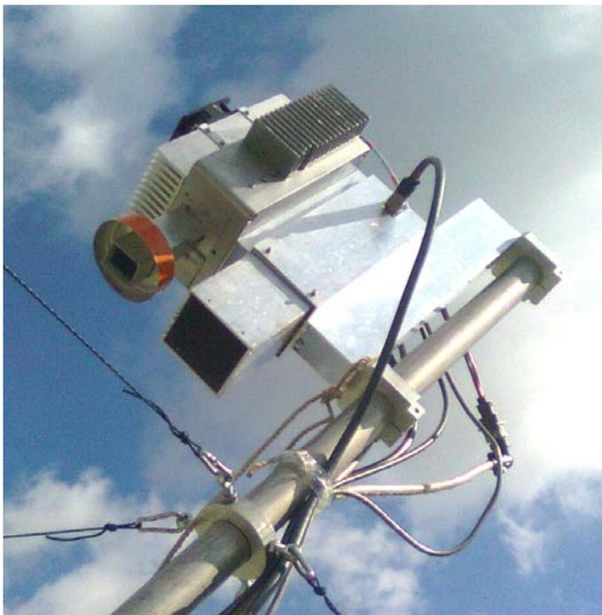
**OKICA's 13 and 6 cm multiband feed arrangement**
