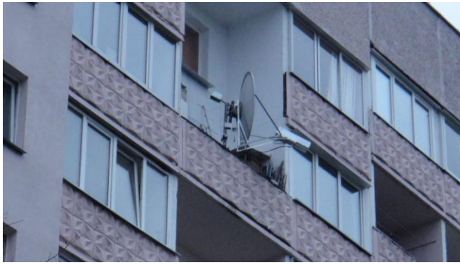
EW1AA's new 1.2 m dish with 1296 septum feed
